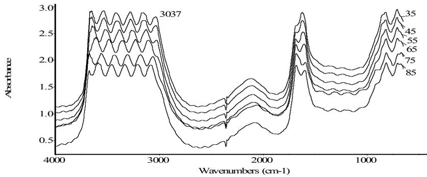
Fig.1. The infrared absorption spectra of pure water and their frequency shifts at different temperatures  $T = 35, 45, 55, 65, 75, 85$ .
