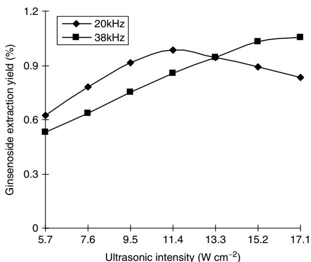
**Figure 5.** Effect of ultrasonic frequency on ginsenoside extraction by USCRME.
