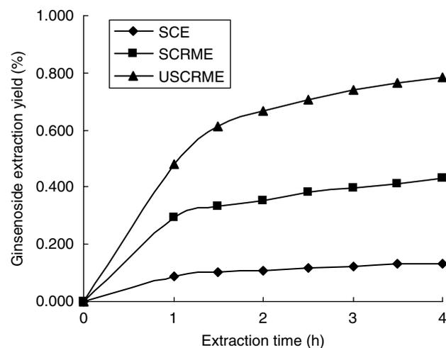
**Figure 2.** Ginsenoside extraction kinetics of SCE, SCRME and USCRME.
