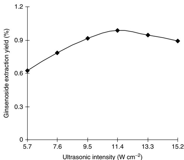
**Figure 3.** Effect of ultrasonic intensity on ginsenoside extraction by USCRMME.
