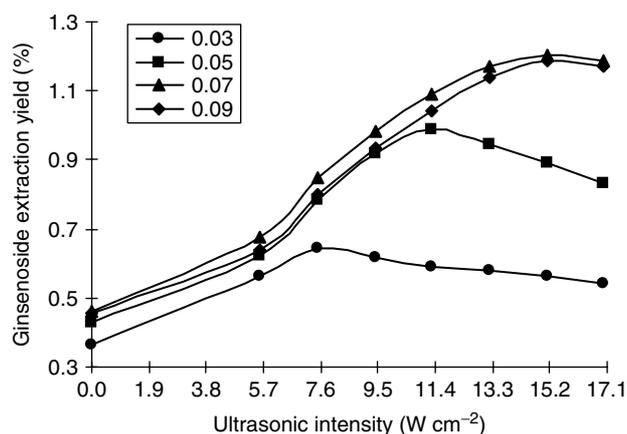
**Figure 6.** Effect of ultrasound on different concentrations of reverse microemulsions in ginsenoside extraction by USCRME.
