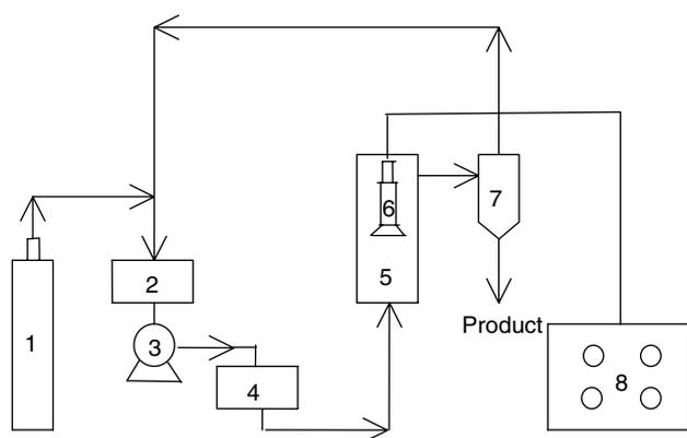
**Figure 1.** Experimental set-up of 1 L ultrasound-enhanced supercritical CO<sub>2</sub> extraction: 1, CO<sub>2</sub> supply; 2, cooler; 3, high-pressure pump; 4, CO<sub>2</sub> storage; 5, extractor; 6, ultrasonic transducer; 7, separator; 8, ultrasonic generator.
